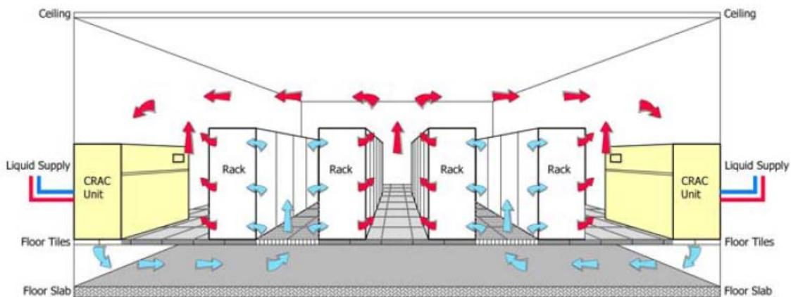
Figure 4. CRAC Unit Deployment
