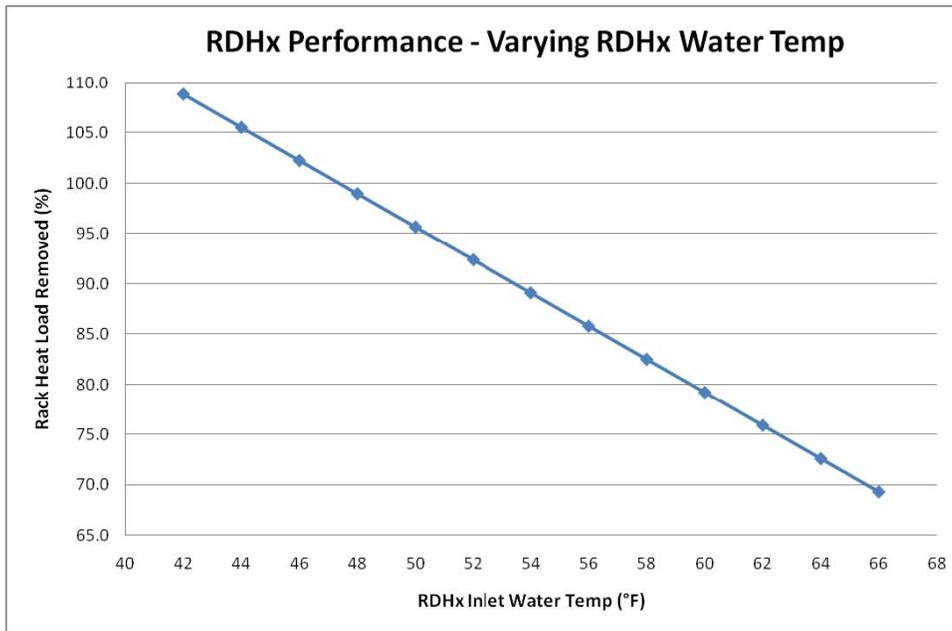
Figure 9. RDHx Performance Sensitivity to Water Temperature
